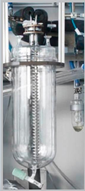
The water removal system is available as an accessory for TBP and Combi plants. It consists of a double mantle glass vessel (collector vessel) with internal quench cooler and bottom drain valve. The vessel can be removed when not in use. The collector vessel can be charged with 5 litre water/distillate mixture. Other sizes, like 10 or 20 litre (for large TBP's) are also available.
