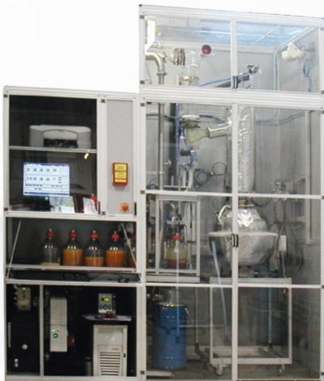
The Potstill-L models have a bigger framework and a movable flask support. For safety reasons and easy access, the big and heavy cold trap is situated close to floor level. The support can swing out, which simplifies any service work.
