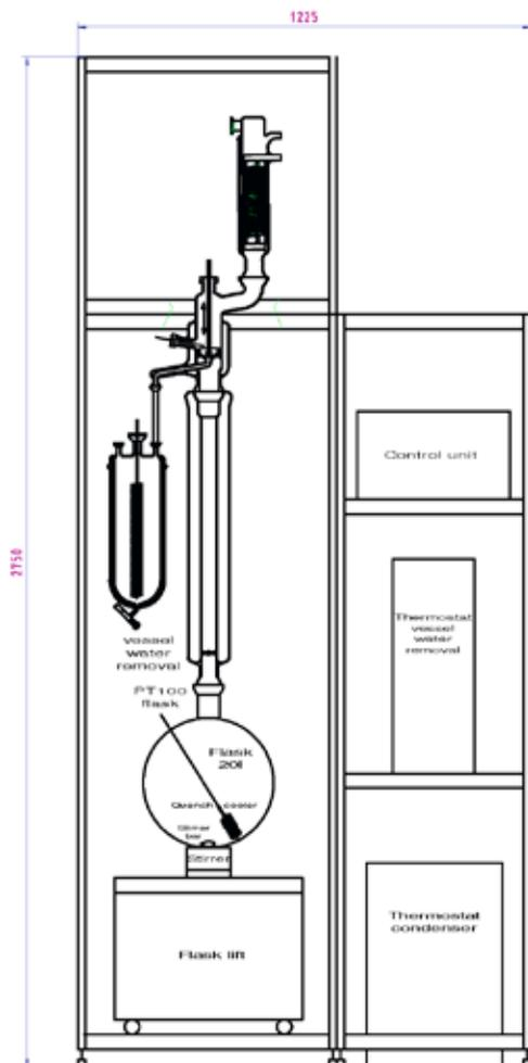
Alternatively, a stand alone water removal system is available. It comes with a complete framework with front doors, a complete set of glassware (condenser, reflux divider and column) and flask heater (with stirrer). The system comes with two thermostats; one for the condenser; one for the collector vessel. The plant has its own control system, which allows an unattended operation.
