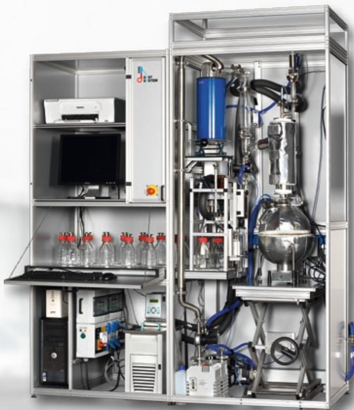
The ASTM D 5236 (Potstill) can fractionize crude oil or crude oil residue from 15°C up to 565 °C (at atmospheric equivalent temperature); from atmospheric pressure down to a vacuum of 0,1 Torr.
