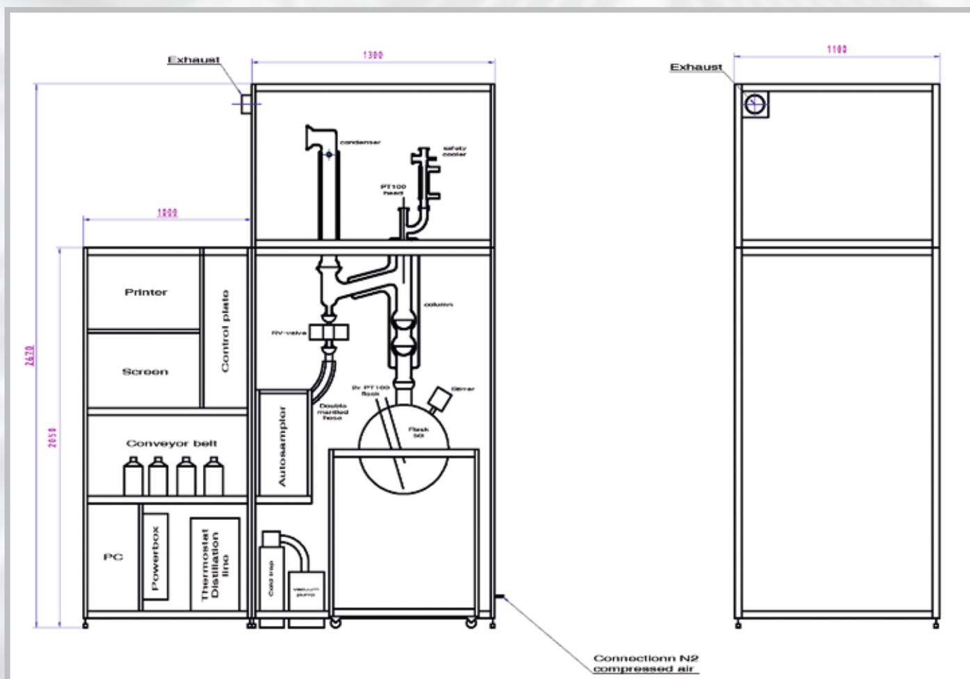
MPS (Mini Potstill) and TBP-M models have the same compact framework design. Thermostats are standing at the rear side and are accessible from the left or right side. The framework stands on rollers. The computer table can be placed at the left or right side.
