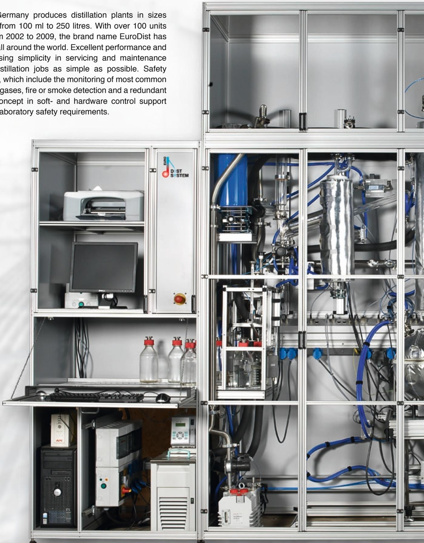
The sophisticated framework concept offers a maximum of flexibility in standard or custom tailored constructions. The framework is constructed modularly, thus fast to assemble or dismantle. Our philosophy is not to hide, but to show all parts of the plant. This allows seeing into the plant function and minimises service time. The plant can stand right in front of a wall; with all services carried out from the front of the unit. Valuable laboratory space can therefore be saved.
