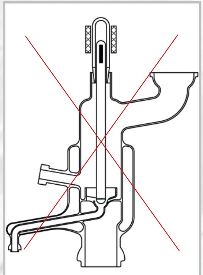
Our reflux divider has a stainless steel or ceramic rod with an O-Ring at the bottom. This O-Ring is pressed into the valve seat with a force of approximately 1 kg and seals the valve with its soft surface.
