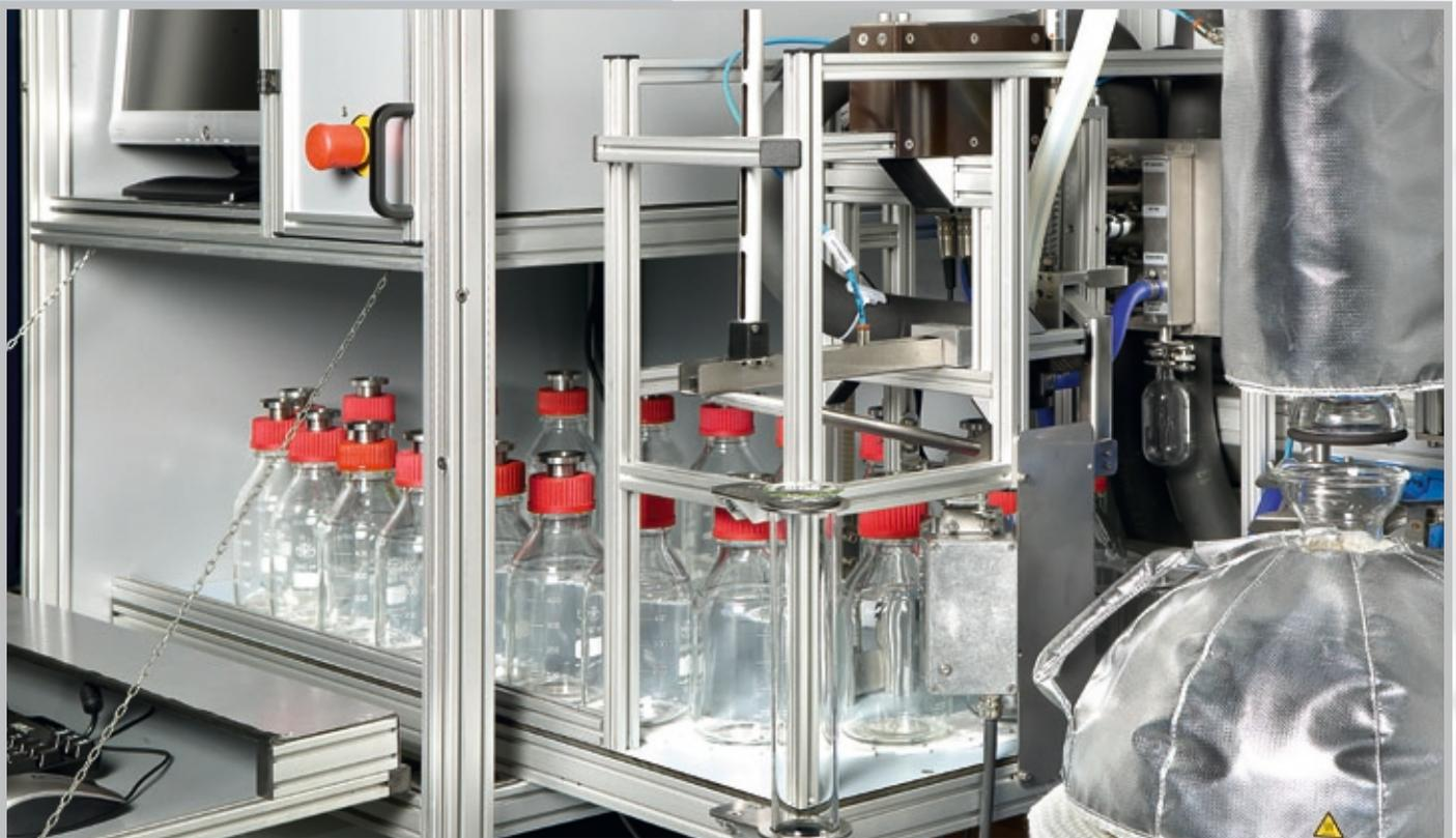
Some customers prefer to have an intermediate receiver. We can supply Standard and Large TBP plants with intermediate receivers of sizes ranging from 250 ml up to 5 litres.
