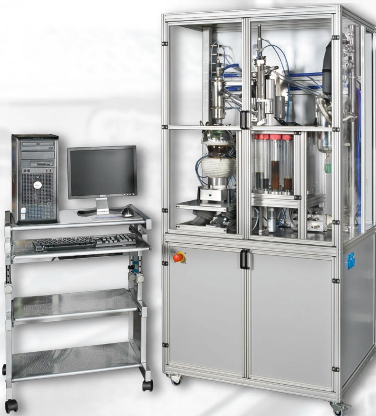
MPS and TBP-M have a carousel, instead of a conveyor belt. The carousel runs within a chamber, which has a front door. The chamber can be heated up to 90°C. It includes a volume follower system, cut weighing equipment and bottle closing.
