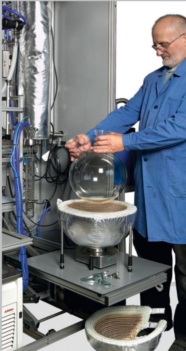
Standing very close to the platform offers a painless charging and discharging of heavy flasks. The platform has a mechanical drive, which can be turned without the need for strength.
