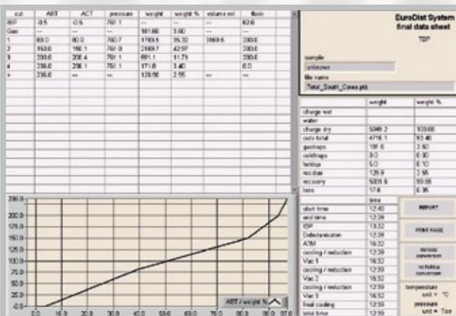
A report of the distillation is generated automatically after distillation. A dialog based program asks user to complete entries for weights ( cold- and gas traps) Data fro TBP and Potstill can be merged to one single report.
