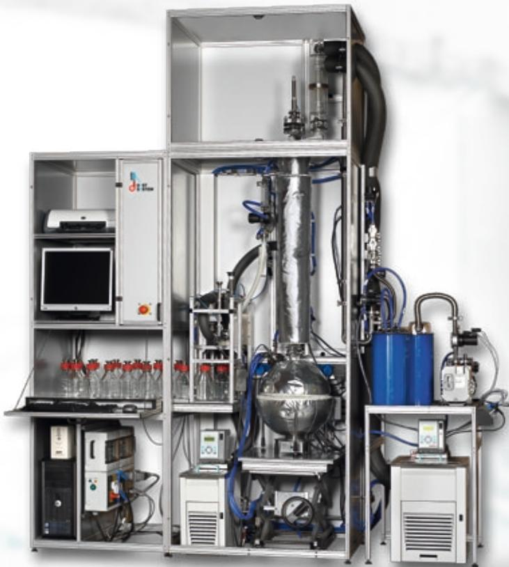
The ASTM D 2892, also called TBP (True Boiling Point) can fractionise crude oils from 15°C up to 420°C AET (atmospheric equivalent temperature) at pressure stages down to 1 Torr.
